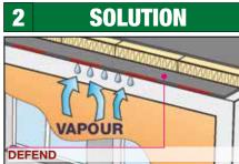
The **DEFEND** Series membranes are used as a vapour barrier layer of thermal insulation materials in construction covers. These membranes consist of non-porous, elastoplastomeric polymer-bitumen which, in itself, is an excellent barrier against vapour migration.
